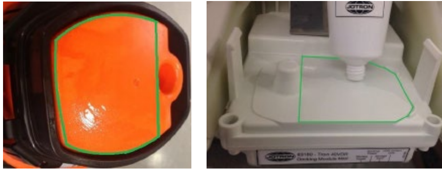
Applying of silicone grease
